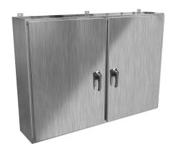
Hammond enclosure, NEMA 3R/4X/12/13, 42 x 60 x 12in (HxWxD), wall mount, 304 stainless steel, #4 brush finish, 2-door, 3-point 316 stainless steel padlocking handle.
