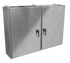
Hammond enclosure, NEMA 3R/4X/12/13, 42 x 60 x 12in (HxWxD), wall mount, 316 stainless steel, #4 brush finish, 2-door, 3-point 316 stainless steel padlocking handle.
