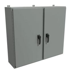
Hammond enclosure, NEMA 3R/4/12, 42 x 48 x 12in (HxWxD), wall mount, carbon steel, ANSI 61 gray, powder coat finish, 2-door, 3-point padlocking handle.
