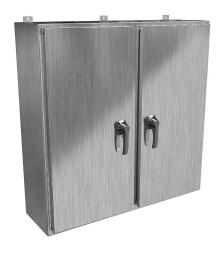
Hammond enclosure, NEMA 3R/4X/12/13, 42 x 42 x 12in (HxWxD), wall mount, 304 stainless steel, #4 brush finish, 2-door, 3-point 316 stainless steel padlocking handle.
