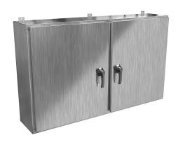
Hammond enclosure, NEMA 3R/4X/12/13, 36 x 60 x 12in (HxWxD), wall mount, 316 stainless steel, #4 brush finish, 2-door, 3-point 316 stainless steel padlocking handle.
