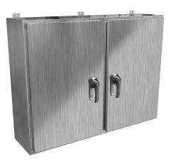
Hammond enclosure, NEMA 3R/4X/12/13, 36 x 48 x 12in (HxWxD), wall mount, 304 stainless steel, #4 brush finish, 2-door, 3-point 316 stainless steel padlocking handle.
