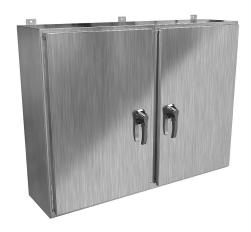
Hammond enclosure, NEMA 3R/4X/12/13, 36 x 48 x 12in (HxWxD), wall mount, 316 stainless steel, #4 brush finish, 2-door, 3-point 316 stainless steel padlocking handle.
