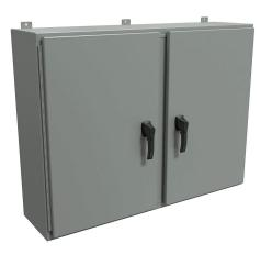
Hammond enclosure, NEMA 3R/4/12, 36 x 48 x 12in (HxWxD), wall mount, carbon steel, ANSI 61 gray, powder coat finish, 2-door, 3-point padlocking handle.
