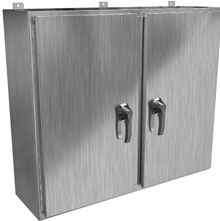
Hammond enclosure, NEMA 3R/4X/12/13, 36 x 42 x 12in (HxWxD), wall mount, 304 stainless steel, #4 brush finish, 2-door, 3-point 316 stainless steel padlocking handle.
