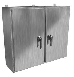
Hammond enclosure, NEMA 3R/4X/12/13, 36 x 42 x 12in (HxWxD), wall mount, 316 stainless steel, #4 brush finish, 2-door, 3-point 316 stainless steel padlocking handle.
