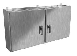
Hammond enclosure, NEMA 3R/4X/12/13, 30 x 60 x 10in (HxWxD), wall mount, 304 stainless steel, #4 brush finish, 2-door, 3-point 316 stainless steel padlocking handle.
