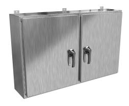
Hammond enclosure, NEMA 3R/4X/12/13, 30 x 48 x 10in (HxWxD), wall mount, 304 stainless steel, #4 brush finish, 2-door, 3-point 316 stainless steel padlocking handle.
