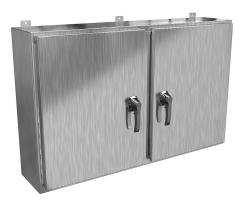
Hammond enclosure, NEMA 3R/4X/12/13, 30 x 48 x 10in (HxWxD), wall mount, 316 stainless steel, #4 brush finish, 2-door, 3-point 316 stainless steel padlocking handle.
