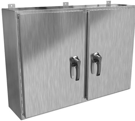
Hammond enclosure, NEMA 3R/4X/12/13, 30 x 42 x 10in (HxWxD), wall mount, 304 stainless steel, #4 brush finish, 2-door, 3-point 316 stainless steel padlocking handle.
