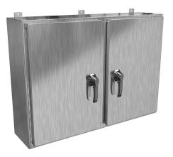
Hammond enclosure, NEMA 3R/4X/12/13, 30 x 42 x 10in (HxWxD), wall mount, 316 stainless steel, #4 brush finish, 2-door, 3-point 316 stainless steel padlocking handle.
