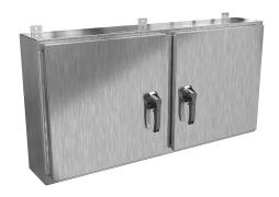
Hammond enclosure, NEMA 3R/4X/12/13, 24 x 48 x 8in (HxWxD), wall mount, 304 stainless steel, #4 brush finish, 2-door, 3-point 316 stainless steel padlocking handle.
