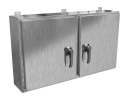
Hammond enclosure, NEMA 3R/4X/12/13, 24 x 42 x 8in (HxWxD), wall mount, 316 stainless steel, #4 brush finish, 2-door, 3-point 316 stainless steel padlocking handle.
