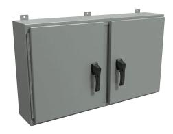
Hammond enclosure, NEMA 3R/4/12, 24 x 42 x 8in (HxWxD), wall mount, carbon steel, ANSI 61 gray, powder coat finish, 2-door, 3-point padlocking handle.
