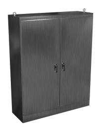
Hammond enclosure, NEMA 3R/4X/12/13, 90 x 72 x 24in (HxWxD), freestanding, 304 stainless steel, #4 brush finish, doubledoor, 3-point 316 stainless steel padlocking handle.
