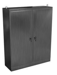
Hammond enclosure, NEMA 3R/4X/12/13, 90 x 72 x 24in (HxWxD), freestanding, dual access, 304 stainless steel, #4 brush finish, double-door, 3-point 316 stainless steel padlocking handle.
