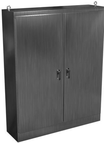
Hammond enclosure, NEMA 3R/4X/12/13, 90 x 72 x 20in (HxWxD), freestanding, 304 stainless steel, #4 brush finish, double-door, 3-point 316 stainless steel padlocking handle.
