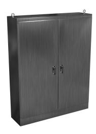
Hammond enclosure, NEMA 3R/4X/12/13, 90 x 72 x 20in (HxWxD), freestanding, 304 stainless steel, #4 brush finish, doubledoor, 3-point 316 stainless steel padlocking handle.
