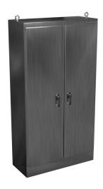
Hammond enclosure, NEMA 3R/4X/12/13, 90 x 48 x 20in (HxWxD), freestanding, 304 stainless steel, #4 brush finish, doubledoor, 3-point 316 stainless steel padlocking handle.
