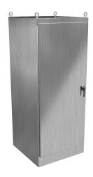
Hammond enclosure, NEMA 3R/4/4X/12/13, 90 x 36 x 36in (HxWxD), freestanding, 316 stainless steel, #4 brush finish, single-door, 3-point 316 stainless steel padlocking handle.
