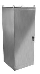
Hammond enclosure, NEMA 3R/4/4X/12/13, 90 x 36 x 36in (HxWxD), freestanding, dual access, 316 stainless steel, #4 brush finish, single-door, 3-point 316 stainless steel padlocking handle.
