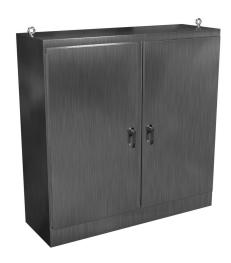
Hammond enclosure, NEMA 3R/4X/12/13, 72 x 72 x 24in (HxWxD), freestanding, 304 stainless steel, #4 brush finish, double-door, 3-point 316 stainless steel padlocking handle.
