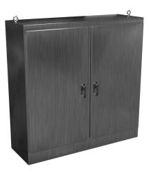
Hammond enclosure, NEMA 3R/4X/12/13, 72 x 72 x 24in (HxWxD), freestanding, dual access, 304 stainless steel, #4 brush finish, double-door, 3-point 316 stainless steel padlocking handle.
