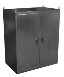
Hammond enclosure, NEMA 3R/4X/12/13, 72 x 60 x 36in (HxWxD), freestanding, 304 stainless steel, #4 brush finish, double-door, 3-point 316 stainless steel padlocking handle.
