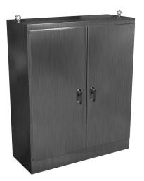
Hammond enclosure, NEMA 3R/4X/12/13, 72 x 60 x 24in (HxWxD), freestanding, 304 stainless steel, #4 brush finish, double-door, 3-point 316 stainless steel padlocking handle.
