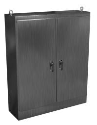
Hammond enclosure, NEMA 3R/4X/12/13, 72 x 60 x 18in (HxWxD), freestanding, 304 stainless steel, #4 brush finish, double-door, 3-point 316 stainless steel padlocking handle.
