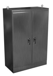
Hammond enclosure, NEMA 3R/4X/12/13, 72 x 48 x 24in (HxWxD), freestanding, 304 stainless steel, #4 brush finish, double-door, 3-point 316 stainless steel padlocking handle.
