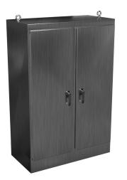
Hammond enclosure, NEMA 3R/4X/12/13, 72 x 48 x 24in (HxWxD), freestanding, dual access, 304 stainless steel, #4 brush finish, double-door, 3-point 316 stainless steel padlocking handle.
