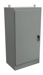
Hammond enclosure, NEMA 3R/4/12/13, 72 x 37 x 24in (HxWxD), freestanding, carbon steel, ANSI 61 gray, powder coat finish, single-door, 3-point padlocking handle.
