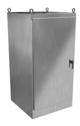
Hammond enclosure, NEMA 3R/4/4X/12/13, 72 x 36 x 36in (HxWxD), freestanding, dual access, 304 stainless steel, #4 brush finish, single-door, 3-point 316 stainless steel padlocking handle.
