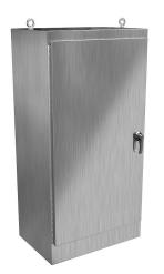
Hammond enclosure, NEMA 3R/4/4X/12/13,  $72 \times 36 \times 24$ in (HxWxD), freestanding, 304 stainless steel, #4 brush finish, single-door, 3-point 316 stainless steel padlocking handle.
