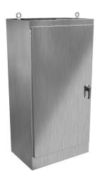
Hammond enclosure, NEMA 3R/4/4X/12/13,  $72 \times 36 \times 24$ in (HxWxD), freestanding, 316 stainless steel, #4 brush finish, single-door, 3-point 316 stainless steel padlocking handle.
