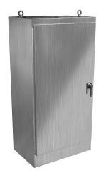
Hammond enclosure, NEMA 3R/4/4X/12/13, 72 x 36 x 24in (HxWxD), freestanding, dual access, 304 stainless steel, #4 brush finish, single-door, 3-point 316 stainless steel padlocking handle.
