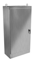
Hammond enclosure, NEMA 3R/4/4X/12/13,  $72 \times 36 \times 18$ in (HxWxD), freestanding, 316 stainless steel, #4 brush finish, singledoor, 3-point 316 stainless steel padlocking handle.
