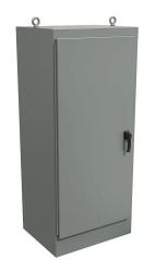
Hammond enclosure, NEMA 3R/4/12/13, 72 x 31 x 24in (HxWxD), freestanding, carbon steel, ANSI 61 gray, powder coat finish, single-door, 3-point padlocking handle.
