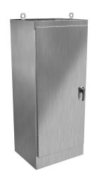
Hammond enclosure, NEMA 3R/4/4X/12/13, 72 x 30 x 24in (HxWxD), freestanding, 304 stainless steel, #4 brush finish, single-door, 3-point 316 stainless steel padlocking handle.
