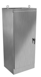
Hammond enclosure, NEMA 3R/4/4X/12/13,  $72 \times 30 \times 24in$  (HxWxD), freestanding, 316 stainless steel, #4 brush finish, single-door, 3-point 316 stainless steel padlocking handle.
