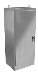
Hammond enclosure, NEMA 3R/4/4X/12/13, 72 x 30 x 24in (HxWxD), freestanding, dual access, 316 stainless steel, #4 brush finish, single-door, 3-point 316 stainless steel padlocking handle.
