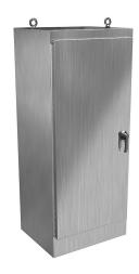
Hammond enclosure, NEMA 3R/4/4X/12/13, 72 x 30 x 24in (HxWxD), freestanding, dual access, 304 stainless steel, #4 brush finish, single-door, 3-point 316 stainless steel padlocking handle.
