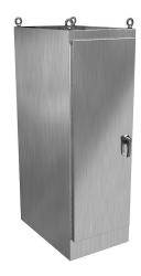
Hammond enclosure, NEMA 3R/4/4X/12/13, 72 x 24 x 36in (HxWxD), freestanding, dual access, 304 stainless steel, #4 brush finish, single-door, 3-point 316 stainless steel padlocking handle.
