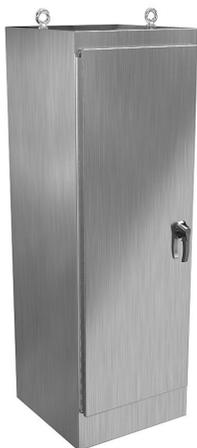
Hammond enclosure, NEMA 3R/4/4X/12/13, 72 x 24 x 24in (HxWxD), freestanding, 316 stainless steel, #4 brush finish, single-door, 3-point 316 stainless steel padlocking handle.
