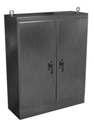
Hammond enclosure, NEMA 3R/4X/12/13, 60 x 48 x 18in (HxWxD), freestanding, 304 stainless steel, #4 brush finish, double-door, 3-point 316 stainless steel padlocking handle.
