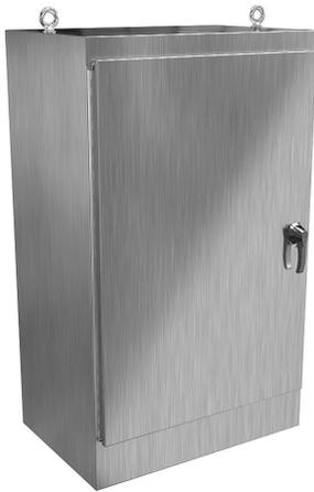
Hammond enclosure, NEMA 3R/4/4X/12/13, 60 x 36 x 24in (HxWxD), freestanding, 304 stainless steel, #4 brush finish, single-door, 3-point 316 stainless steel padlocking handle.
