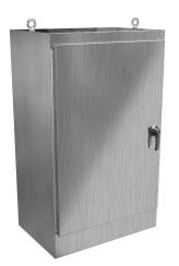
Hammond enclosure, NEMA 3R/4/4X/12/13, 60 x 36 x 24in (HxWxD), freestanding, 304 stainless steel, #4 brush finish, single-door, 3-point 316 stainless steel padlocking handle.
