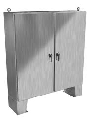
Hammond enclosure, NEMA 3R/4X/12/13, 72 x 72 x 18in (HxWxD), floor mount, 304 stainless steel, #4 brush finish, 2-door, 3-point 316 stainless steel padlocking handle.
