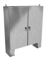
Hammond enclosure, NEMA 3R/4X/12/13, 72 x 72 x 18in (HxWxD), floor mount, 316 stainless steel, #4 brush finish, 2-door, 3-point 316 stainless steel padlocking handle.
