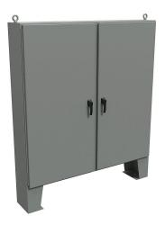
Hammond enclosure, NEMA 3R/4/12/13, 72 x 72 x 12in (HxWxD), floor mount, carbon steel, ANSI 61 gray, powder coat finish, 2-door, 3-point padlocking handle.
