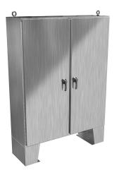
Hammond enclosure, NEMA 3R/4X/12/13, 72 x 60 x 18in (HxWxD), floor mount, 304 stainless steel, #4 brush finish, 2-door, 3-point 316 stainless steel padlocking handle.
